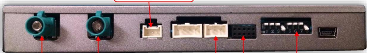
Video OUT (to screen) Video IN (from radio) HDMI Audio OUT IR Eye Not Used Dip Switches
