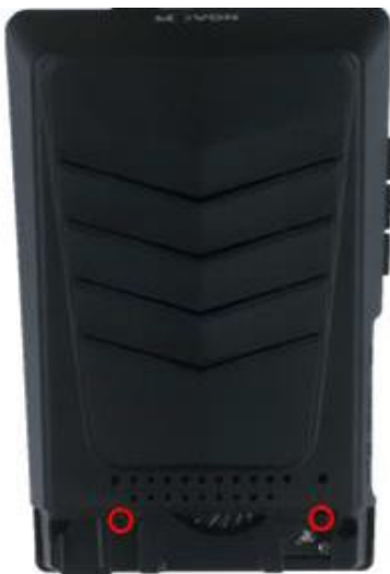
2. Remove (2x) screws, remove plastic cover
