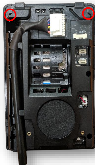
3. Remove (2x) screws, pry plastic mounting frame off unit from corners
