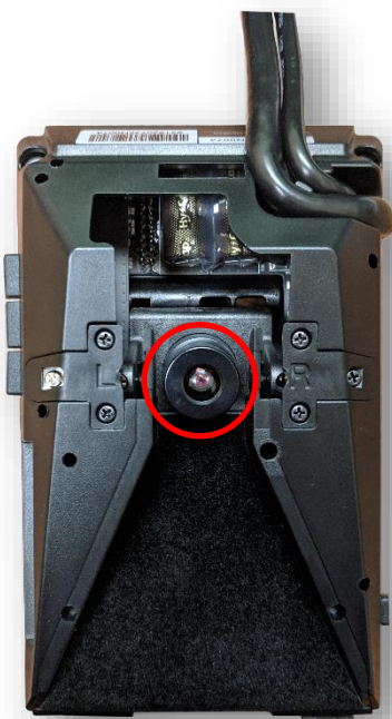
5. Press tightly into channels when routing cables. Remove front camera dust sticker.
