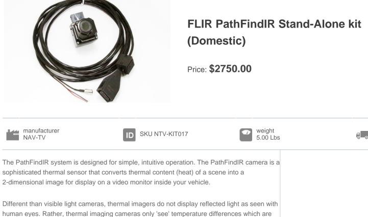
converted into shades of grey, from black to white. The PathFindIR camera displays cold objects as black and hot objects as white.
